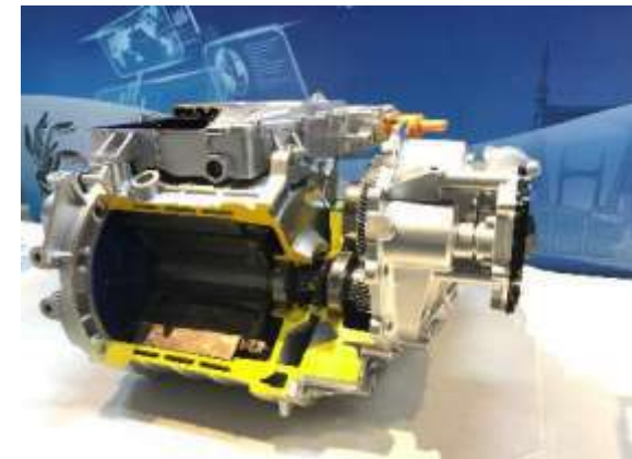
Efficiency of the "three-in-one" drive reaches 97%, noise in full operation less than 80dB
